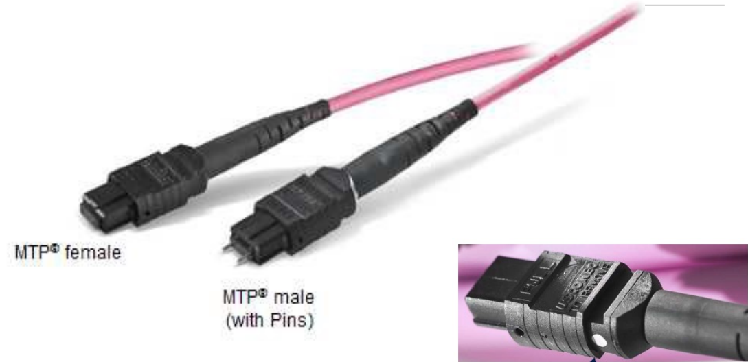
The fiber positions within MTP® connectors are counted from the side with the white mark.
