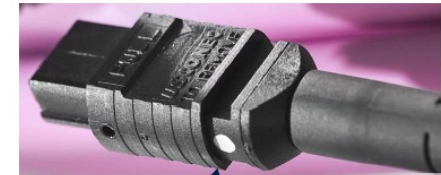
The fiber positions within MTP® connectors are counted from the side with the white mark.
