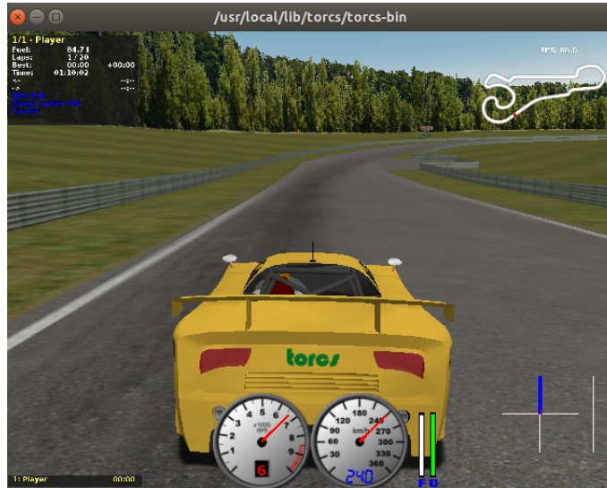
Figure 4.3: TORCS is an open-source racing car simulator that supports controlling the vehicles with custom algorithms.
