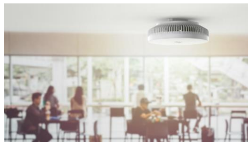
Figure 12. Radio Dot, mounted on the ceiling (source: [46])
