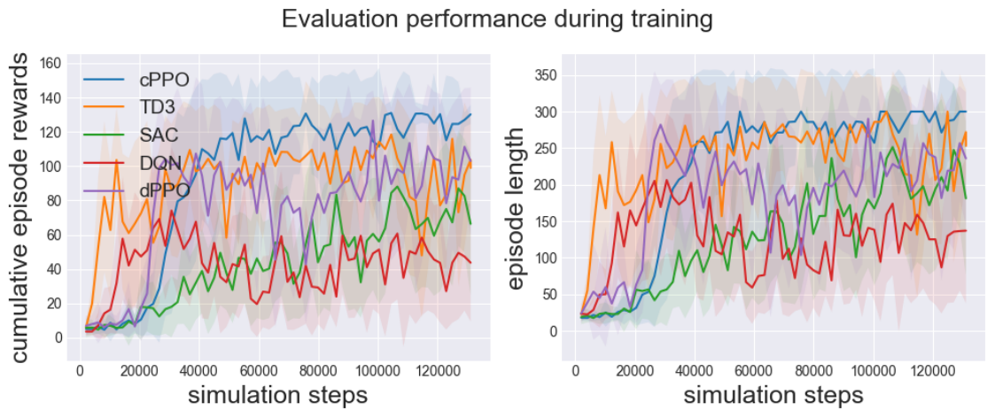
Figure 25: Comparison of RL algorithms in the custom lane following environment. cPPO and dPPO mean PPO algorithms with continuous and discrete action spaces, respectively.
