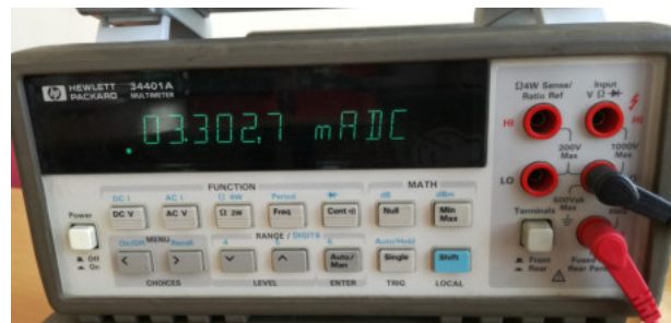
Figure 5.16: Measurement of the current generator - upper limit
