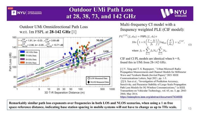
Figure 3. Research shows path loss at frequencies above 100 GHz differs little from path loss at mmWave frequencies. Source: NYU Wireless
