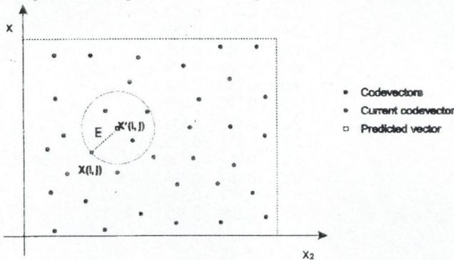
Fig. 1. The basic idea of DCR vector quantization
