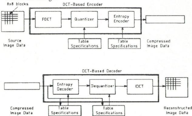
Fig. 7. JPEG compression and decompression
