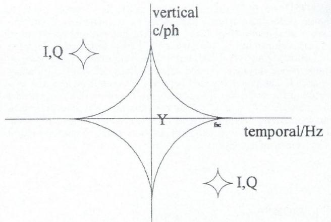
Fig. 1(c). NTSC vertical/temporal frequency spectrum
