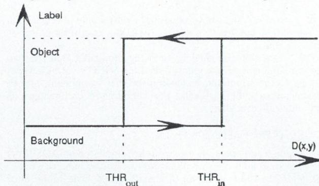
Fig. 3. Graphic representation of the hysteresis function used
