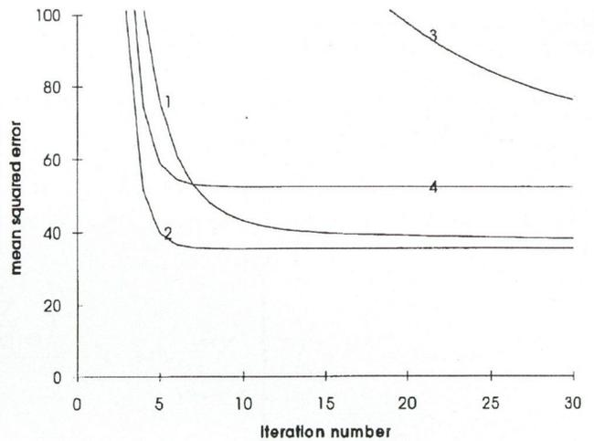
Fig. 6. Comparison of the conventional and the modified 1<sup>st</sup> order luminance transformation: conventional: 1 non-quantized, 3 quantized, modified: 2 non-quantized, 4 quantized
