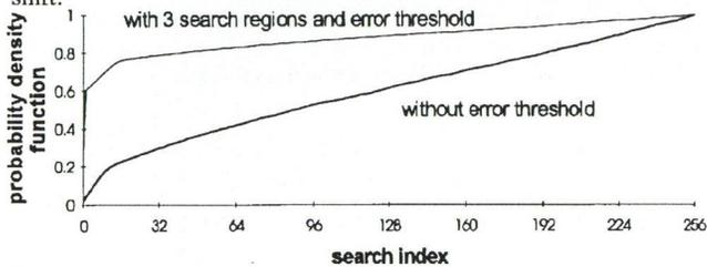
Fig. 2. Probability density function of the geometrical codebook indices using a search scheme as shown in Fig. 3. The maximum search region was 8 bit. The additional search regions used a search width of 0 and 4 bits.
