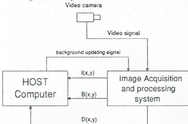
Fig. 2. The image acquisition module
