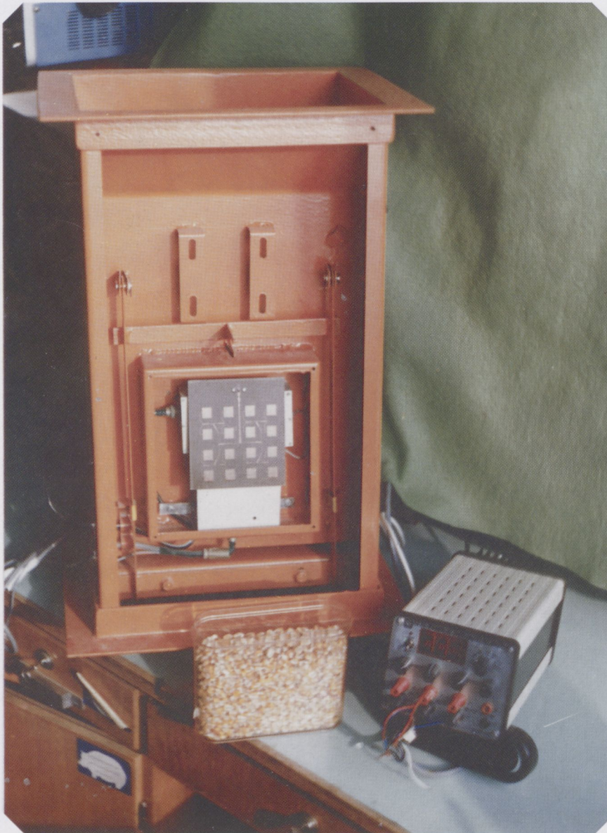
Fig. 26. Upper part: Dual-polarized X-band scatterometer MSA-array, having two independent inputs (SMA-connectors are behind the back-metallization). Lower part: turned-out MSA-array of the moisture sensor for corn [10].
