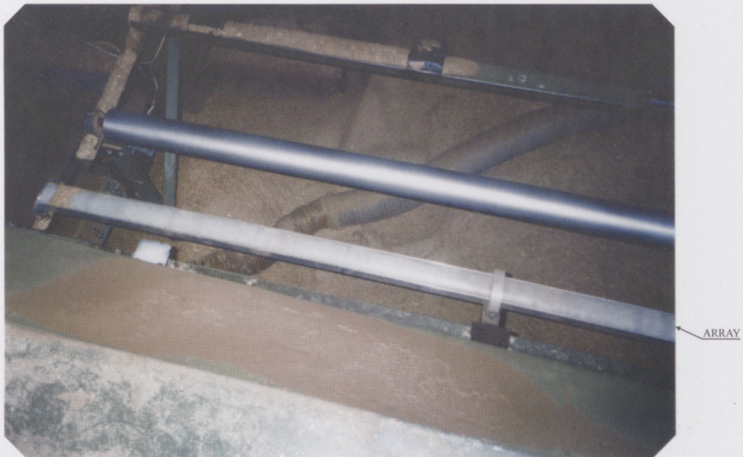
Fig. 25. On the top: circularly polarized Tx/Rx antennas for on-line monitoring of particleboard production [22]. On bottom: backscatterer array of dual-element BPSK-modulators (see Fig. 23.), as it shown on the lower part of the photograph
