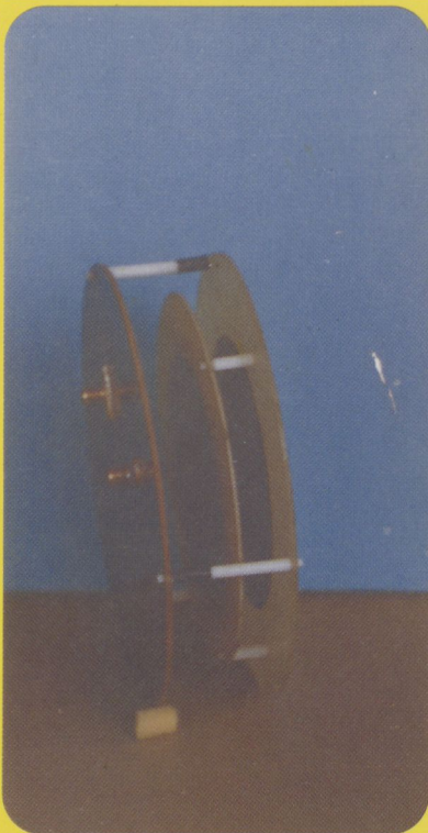
Fig. 14. Different types of experimental MSAs [13] made at TUB/DMT. Travelling-wave (meander line) antennas, single- and multilayer resonant arrays realized on plastic substrates (Polyguide, Duroid) and on ceramic (alumina) are shown on photograph in right side. On the top a three-layer, dual-polarized circular patch with parasitic elements is shown. Circularly polarized meander-line antenna array with four inputs is shown on the left-bottom.
