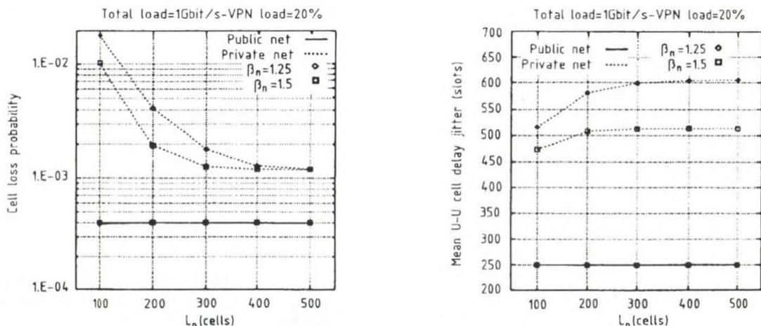
Fig. 9. Diagrams of cell loss probability and End-to-End delay versus  $L_n$  and  $\beta_n$ . The figure is referred to the case where a two-level (users and network) shaping function is implemented on the private traffic.
