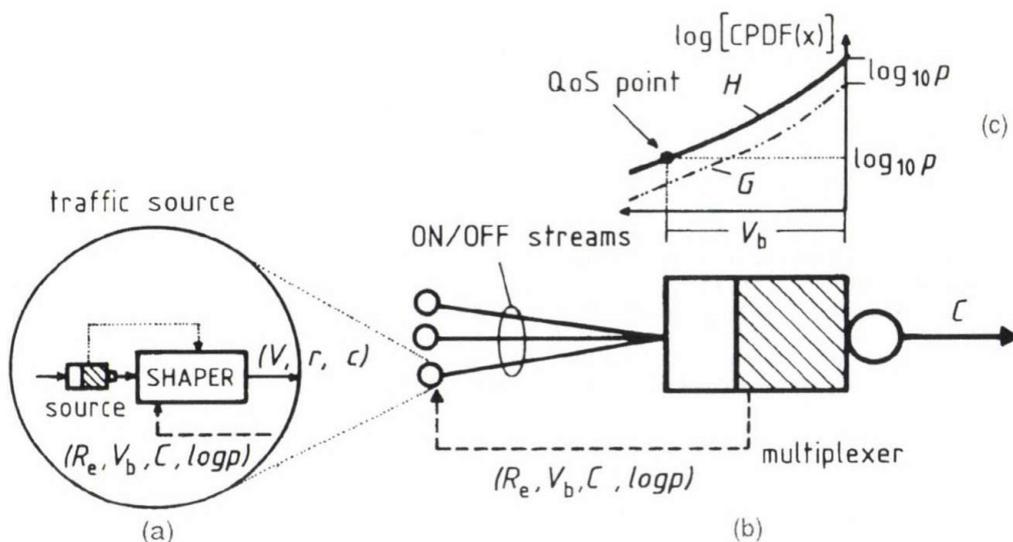
Fig. 1. An ATM statistical multiplexing environment. (a) traffic sources with adaptive shaping capabilities; (b) multiplexer; (c) complementary distribution of buffer occupancy
