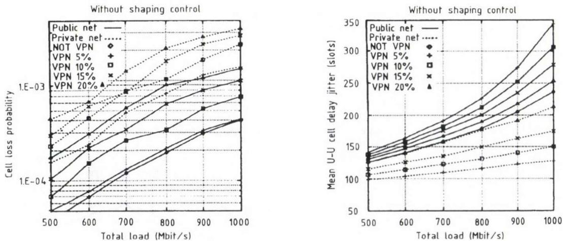
Fig. 3. Diagrams of cell loss probability and End-to-End delay versus total network load and private network load percentage. The figure is referred to the case where no control exists on the private traffic.
