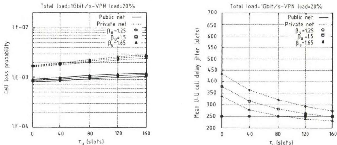
Fig. 4. Diagrams of cell loss probability and End-to-End delay versus  $\beta_u$  and  $\tau_u$ . The figure is referred to the case where a shaping function is implemented at each private user's premise.
