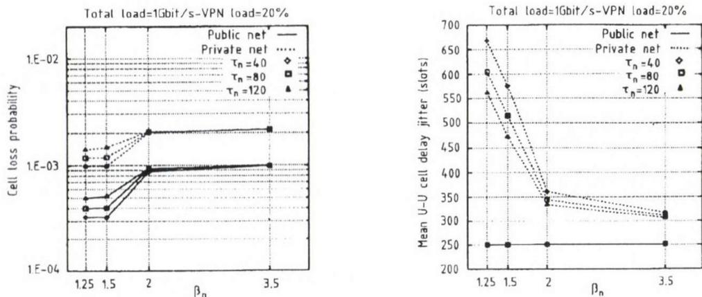
Fig. 7. Diagrams of cell loss probability and End-to-End delay versus  $\beta_n$  and  $\tau_n$ . The figure is referred to the case where a two-level (users and network) shaping function is implemented on the private traffic.
