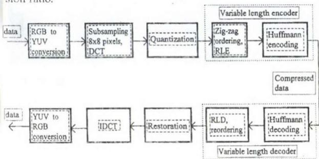
Fig. 1. The JPEG standard algorithm's baseline structure
