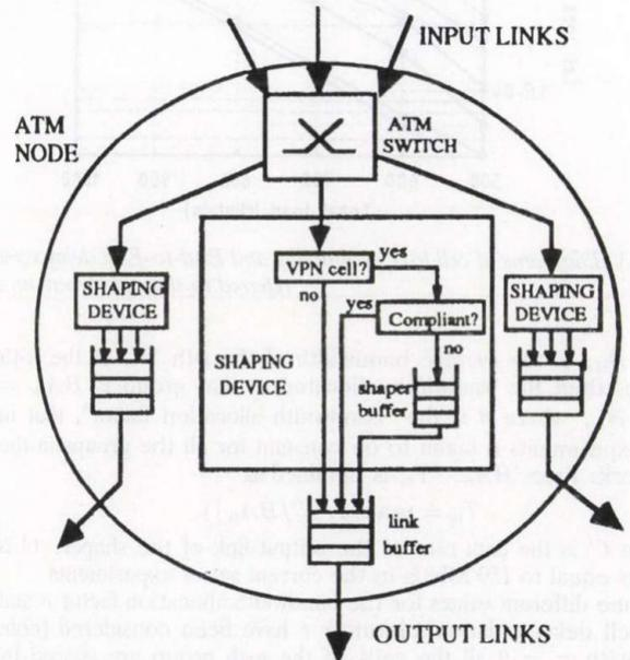
Fig. 5. Architecture of the traffic shaping mechanism implemented inside the ATM network.
