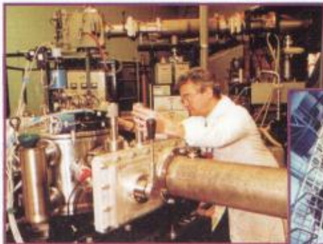
Non-destructive compositional and structural analysis by means of ion beam techniques, BS/C, ERD, NRA (5 MV Van der Graaf accelerator, joint chamber with 400 kV heavy ion implanter)
