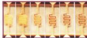
Porous silicon bulk micromachined filaments for explosive gas detection array (FW5 SAFEGAS Project).
