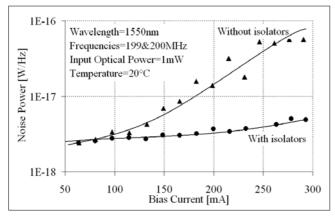
Figure 10. Noise level depends on the optical reflection
