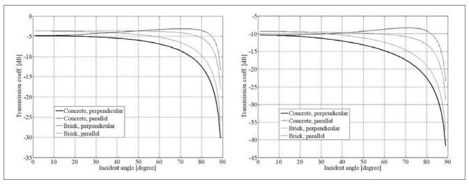
Figure 3. Transmission coefficients at 900 MHz and 2.4 GHz
