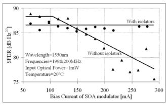
Figure 9. SFDR depends on the optical reflection
