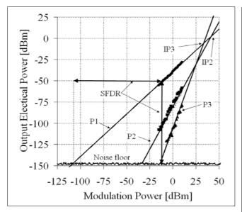
Figure 6. Determination of SFDR, IP2, IP3
