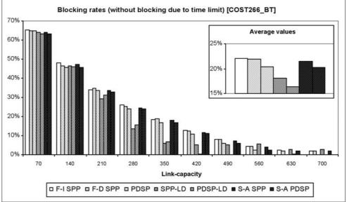
The topology characteristics of network COST266\_RT (low graph-connectivity, low average focal degree) make it suitable to demonstrate the weaknesses of path protection. If we take a look at *Figure 4*, and focus on the low-blocking capacity-range, a significant difference is noticeable between the segment and path-protection methods.
