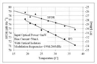
Figure 8. Nonlinearity depends on the Temperature
