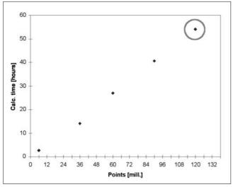
Figure 20. Running time requirement of simulation
