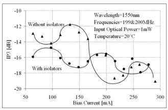
Figure 11. Nonlinearity depends on the optical reflection
