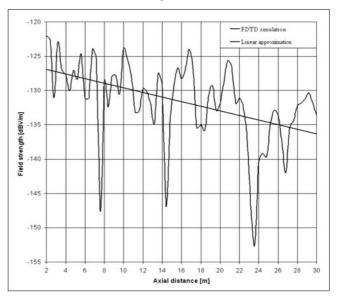
Figure 15. Field strength distribution of radial plane in tunnel without and with vehicle
